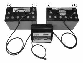
Connect a heavy duty UL approved extension cord to the power cord of your charger and then plug the extension cord into a nearby 120VAC GFI protected (Ground Fault Circuit Interrupt) outlet. You should now observe a red LED indication on each bank of the charger representing each individual battery being charged. The voltage of each battery will reflect the number of LED indicators illuminated.
