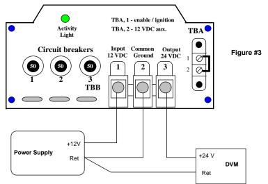
b) Make sure terminals 1 & 2 on TBA are shorted and that the Power supply is turned off. Set the DVM to the appropriate scale to read 24 VDC at the desired accuracy.
