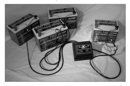
Locate the purple wire at the end of the starting battery cable assembly. Using the supplied quick connector, attach the purple wire to any 12 volt source on the boat that is disabled when the boat is not in use. The purpose for this connection is to disable the ProXtra circuitry during times that the batteries may be charged by other means. (i.e. AC powered battery charger)
